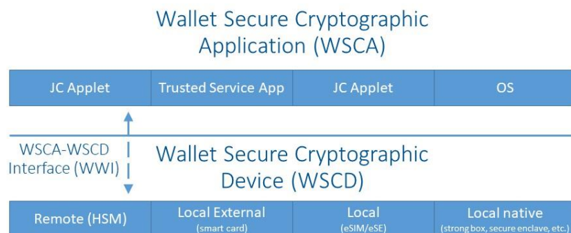
Figure 1: Wallet Secure Cryptographic Devices and Applications - Extracted from the ARF Version 1.5 7
