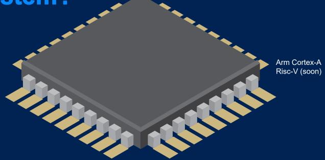
Larger "microprocessors" used in larger ECUs and domain, or zonal, controllers typically DO have the hardware capabilities for a TEE and TEE Operating Systems are common.
