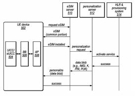
resolved by Apple's eSIM Server and ultimately by the MNO's HLR. In order to implement this architecture Apple need to interface with the MNOs backend APIs HLR and Authentication Centre (AuC) to be able to register and authenticate the subscriber on the network. After this provisioning has occurred, the eSIM provisioning is complete, and the handset should be able to attach to the MNOs network.
