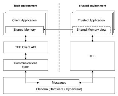
Figure 2-1: TEE Client API System Architecture
