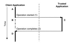
Figure 3-2: Memory Reference timing diagram
