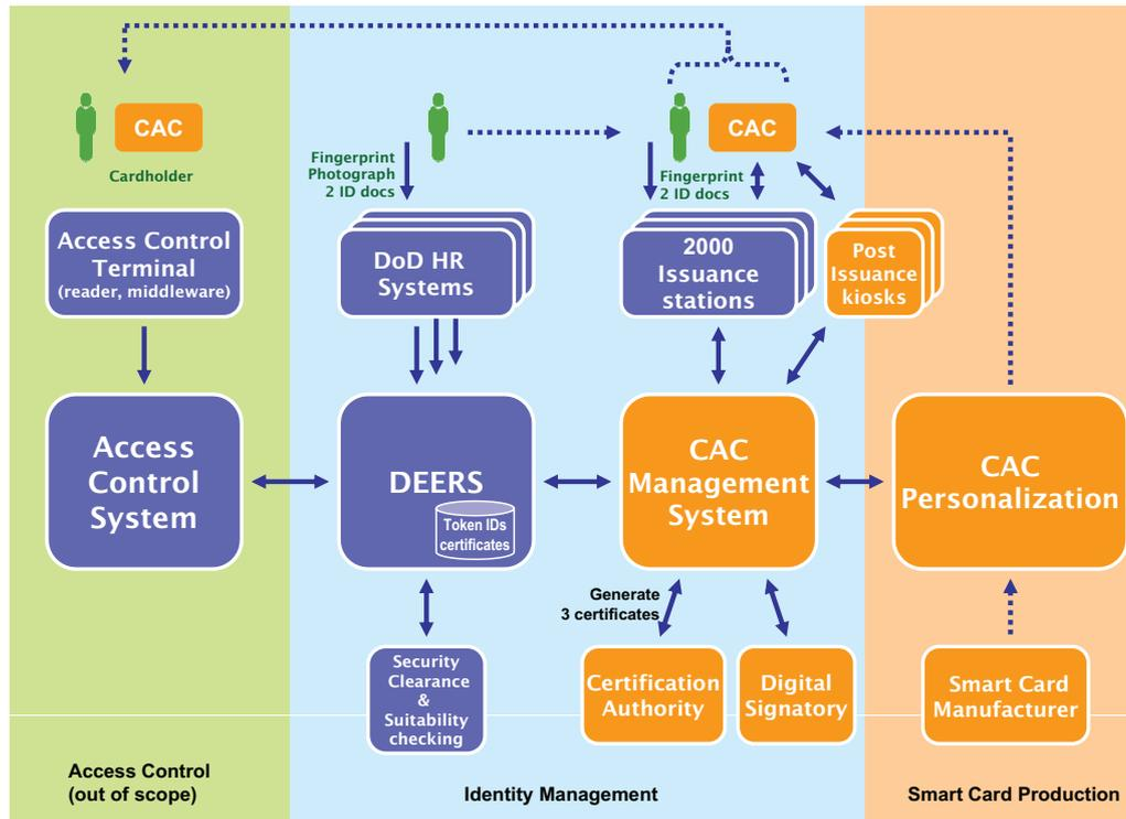
**Figure 4 - A conceptual overview of the Common Access Card (CAC) system concept**
