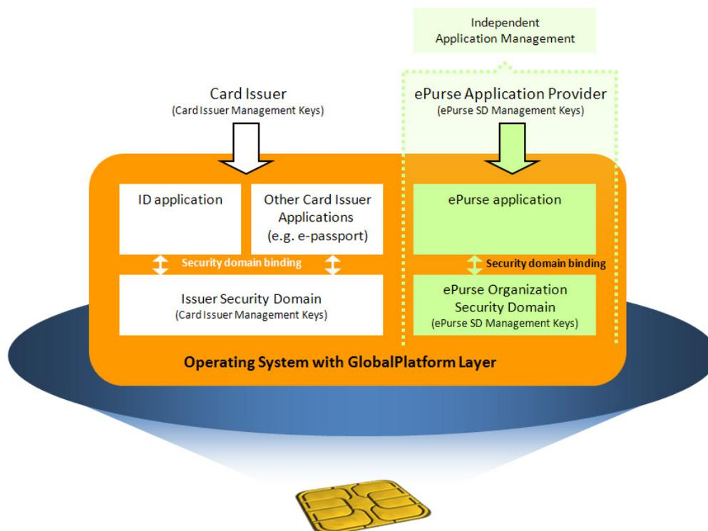
**Figure 7 – GlobalPlatform offers the issuer a means to give application providers their own Security Domains on the chip, while assuring that applications, application data and application management remain totally separate**
