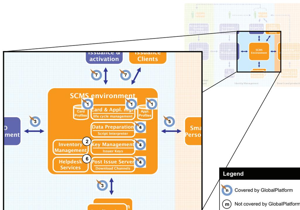
**Figure 12 – The functional components of the Smart Card Management System (SCMS) environment according to GlobalPlatform**
