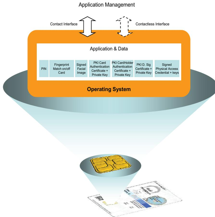
**Figure 5 – Card issuers need a uniform mechanism to load, update and delete applications on the chip**
