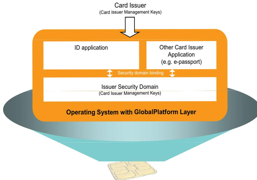
**Figure 6 – GlobalPlatform has defined a standardized mechanism by which issuers own a Security Domain, providing them with a Secure Channel to manage applications on the chip**
