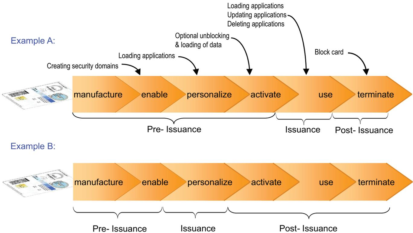
**Figure 8 - Typical life cycle phases of a smart card**
